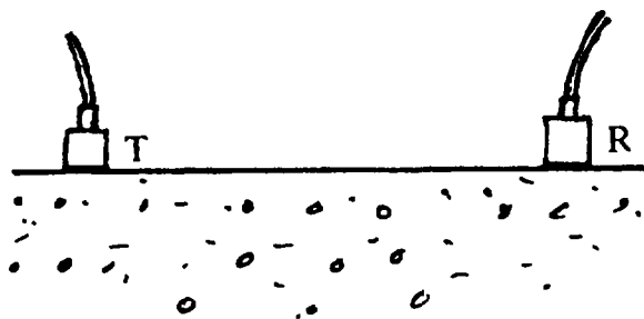
Figure 6.61 (c) : Indirect or surface transmission.
