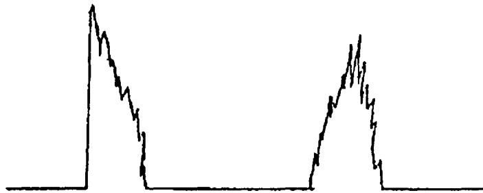
Figure 8.17 : Shape of echo from a slag inclusion.
