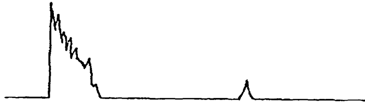
Figure 8.15 : Shape of the echo from a pore.
